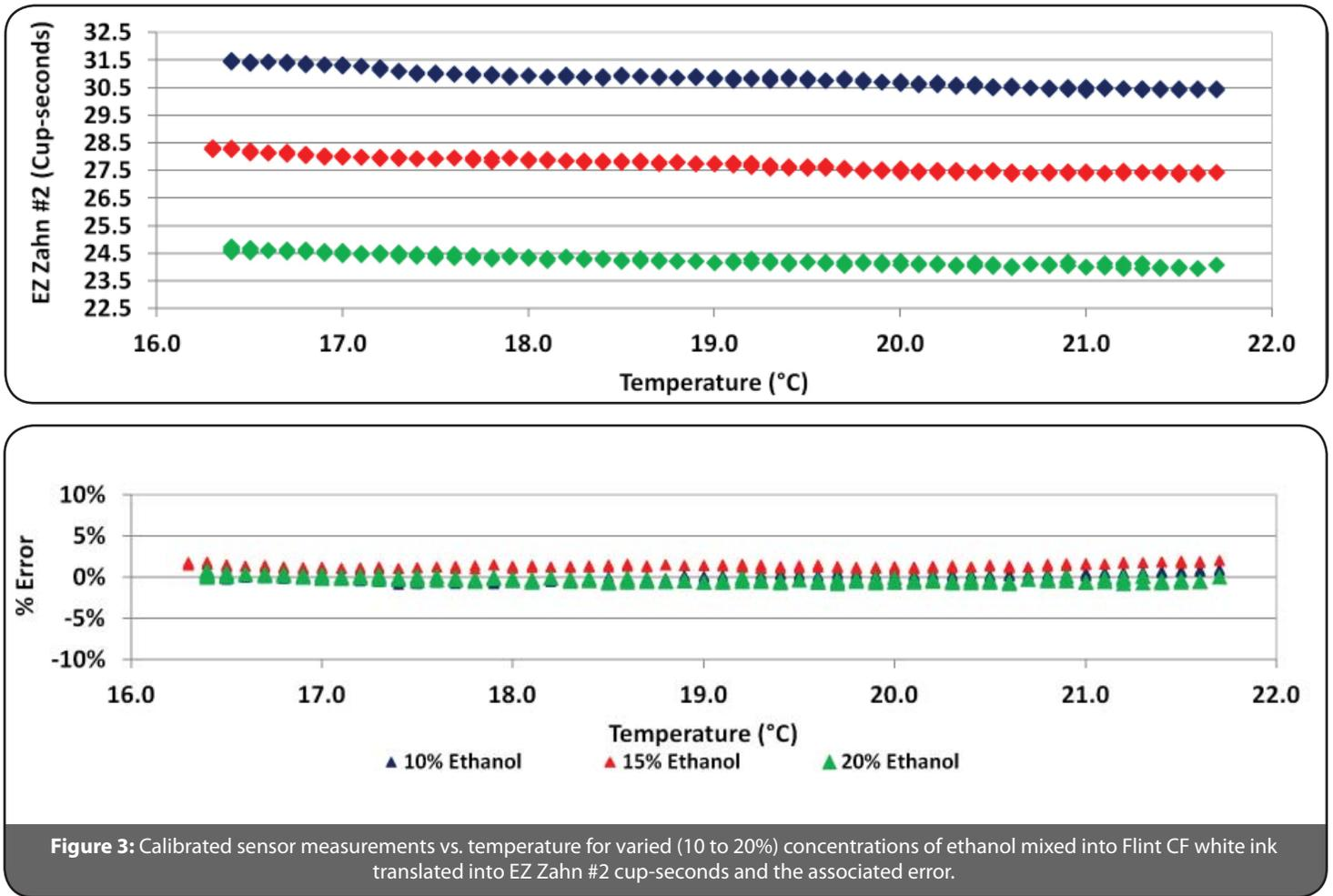
**Figure 3:** Calibrated sensor measurements vs. temperature for varied (10 to 20%) concentrations of ethanol mixed into Flint CF white ink translated into EZ Zahn #2 cup-seconds and the associated error.
