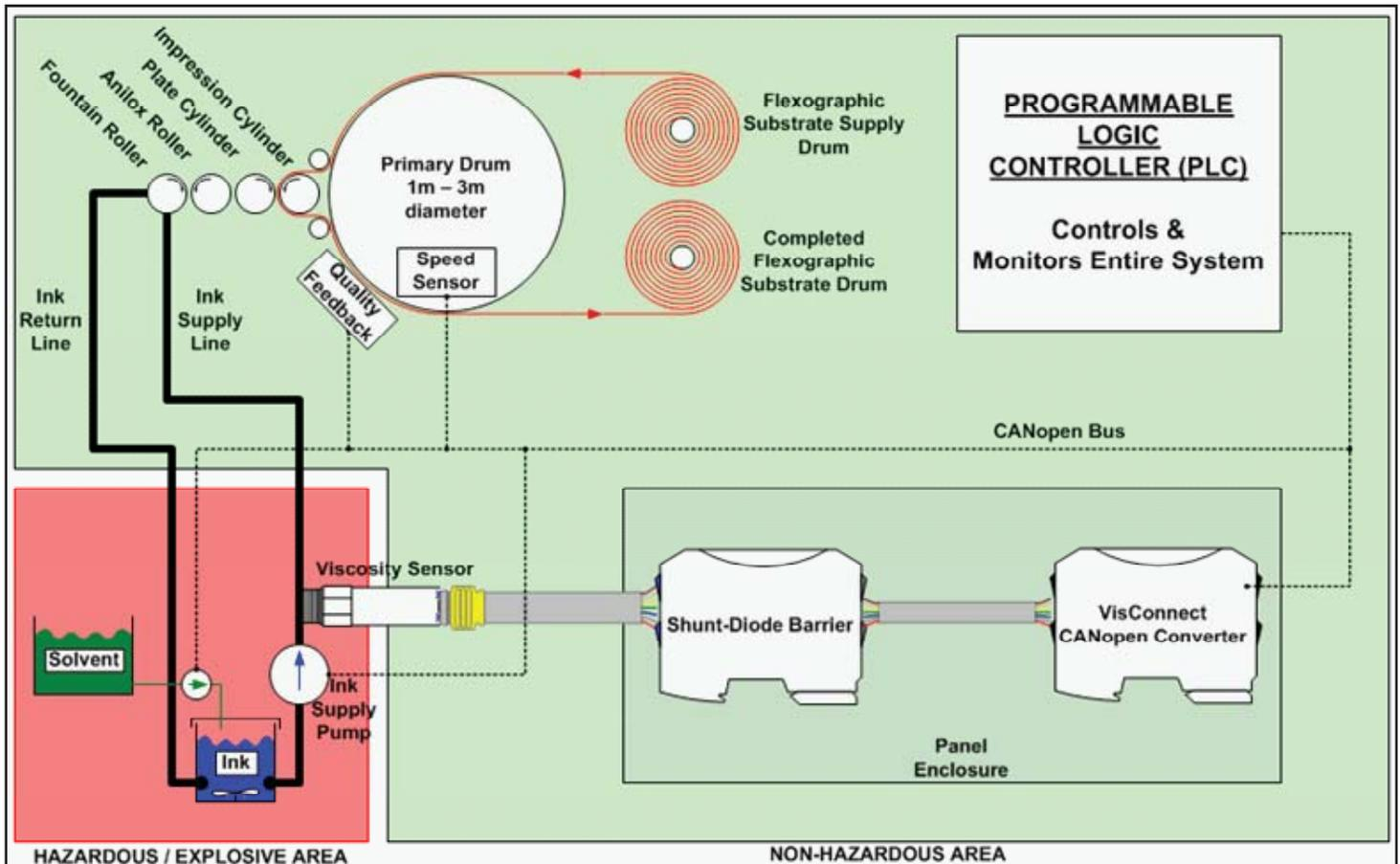
Figure 3: Mounted in-line with the ink supply line, the solid-state viscosity sensor provides continuous viscosity measurement of ink to allow real time control of ink viscosity.
