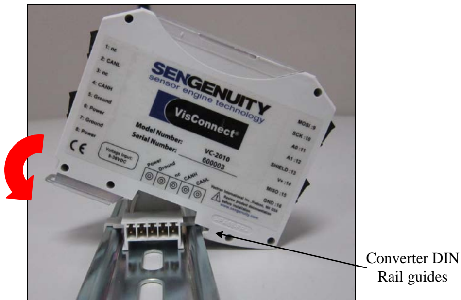
Figure 2: Converter Installation on DIN Rail
